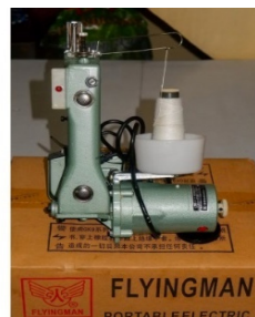
Bag closer sewing machine with polyester fabric rope
